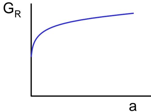
Static delamination R-curve
