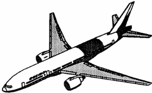
*An equivalent metal fuselage section has 10 panels*
